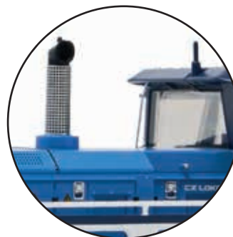
Exhaust pipe panelling made from photo-etched
