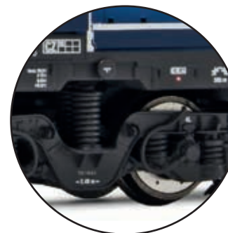
Fine detailed bogies with metal brake discs
